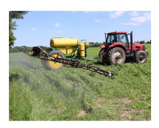
If the pressure remains constant, then halving ground speed will double output, and doubling ground speed will halve output. If ground speed remains constant, then quadrupling pressure will double output, and quartering pressure will halve output.
