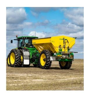
If the feed gate opening remains the same, then halving ground speed will not affect output, and doubling ground speed will also not affect output. If ground speed remains constant, then doubling the rate of granules released from the feed gate with a larger opening will double the output, and halving the rate of granules released from the feed gate with a smaller opening will halve the output.
